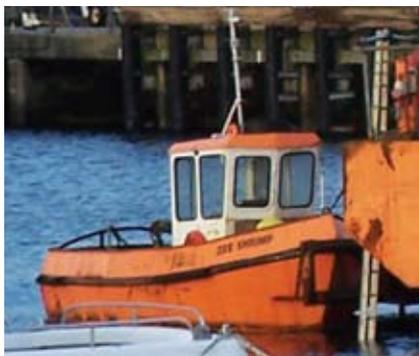
Our 120-hp Zee Shrimp safety boat has been designed to be highly transportable. It can be fully equipped as a nearshore/inshore workboat and is an ideal small tug for manoeuvring the Zee Jack Inspector jack-up platform in sheltered waters.
