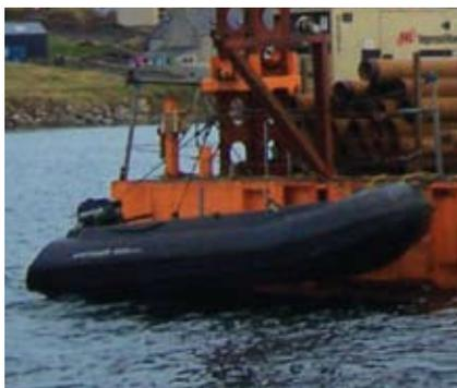
Made from rotational-moulded polyethylene, the Steady 400 has a 1000-kg capacity, will plane at 10 knt while producing very little wake and is extremely manoeuvrable. Its five-person capacity makes this versatile boat ideal for a range of applications, particularly in sensitive environments.
