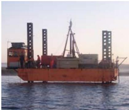
A purpose-built jack-up system, the Zee Jack Inspector provides a stable, elevated environment that supports conventional static drilling and in situ testing in water depths to 25 m. The 10 × 12 × 2-m jack-up platform is fully road demountable for ease of transport and rapid deployment. The jack-up system comes complete with a Steady 400 safety boat and can be fitted with a deck-sited welfare unit.
